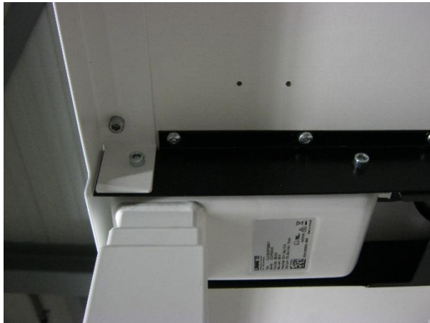
Photo 5: Tested sample 240276-1 of Hi Tee zit-sta duo werkplek 160x80 cm - attachment of horizontal part to vertical part table leg
