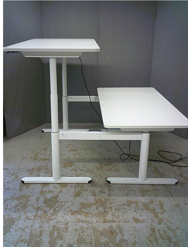
Photo 2: Tested sample 250404-1 of Voortman office desk - side view one table top lowest position other table top highest position.
