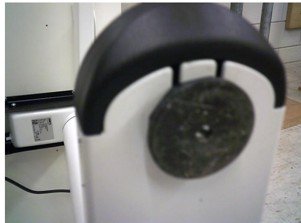
Photo 4: Tested sample 250404-1 of Voortman office desk - detail glider.
