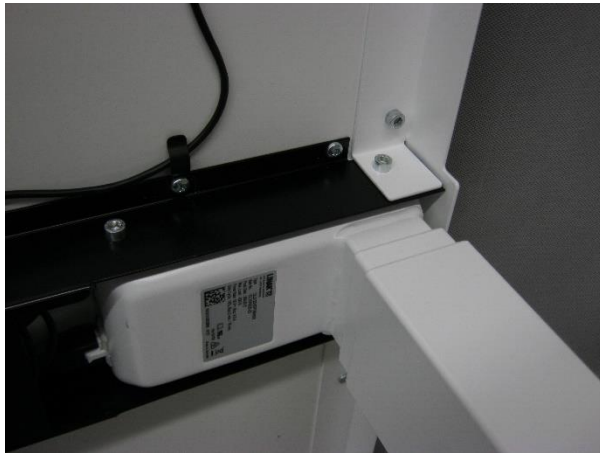
Photo 5: Tested sample 240276-2 of Hi Tee zit-sta bureautafel 160x80 cm - attachment of horizontal part to vertical part table leg
